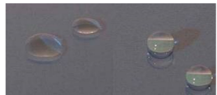
Photo above shows both a non-coated surface and a coated hydrophobic surface.
